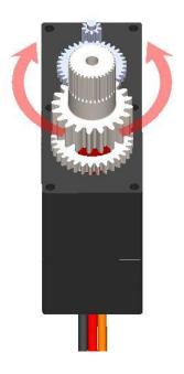
STEP 11: Install the Lynx center metal gear sliding the set in sideways.
