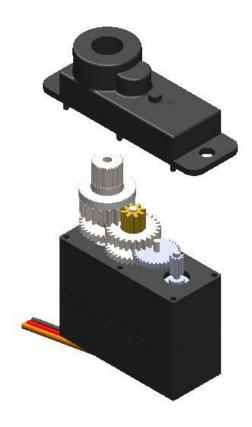
After finishing the servo assembly, test the servo for proper functions. Lynx suggest use a standard servo tester and run a full servo test.
